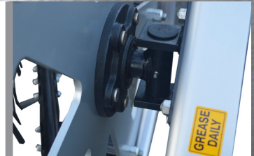
SELF-ALIGNING IDLER HUBS
