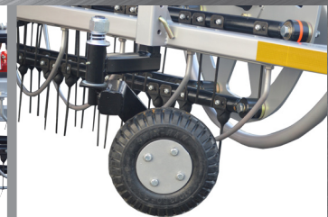
OPTIONAL GAUGE WHEELS w/ TORSION AXLE SUSPENSION
