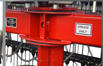
HEAVY-DUTY BASKET PIVOT w/ UHMW SHIMS -SHEAR BOLT PROTECTED
